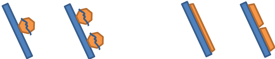
Figure 3.18: Effect of capacity for disintegration by a shock wave (left) versus disintegration by compression into a pancake (right).
