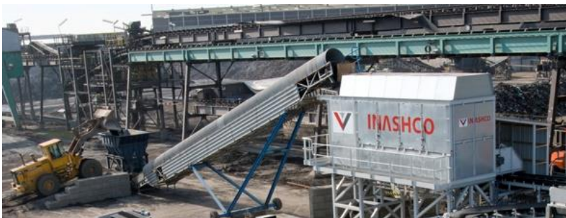
Figure 4.29: Early industrial ADR prototype
