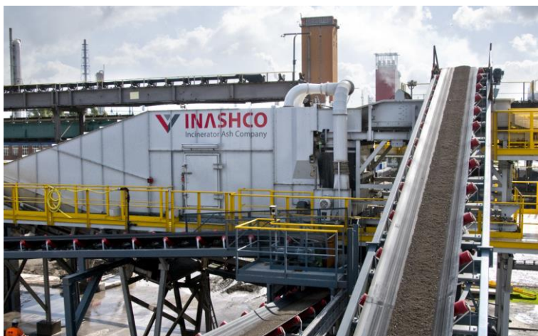
Figure 4.19: Industrial ADR operating at 120 t/h
