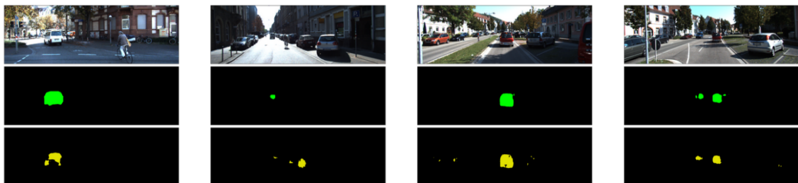
Figure 5.4: Moving object segmentation - Row (i) RGB image (ii) Ground truth (iii) segmentation result
