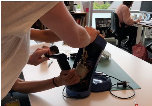
Figure 24: Disassembling a Senseo
