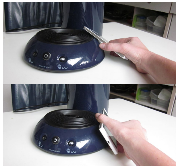
Figure 76: Strange phone angle to scan the tag (top) versus if the tag would be placed more towards the front (bottom)
