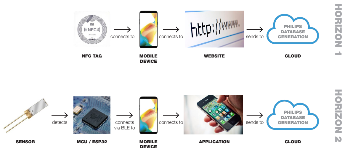
Figure 56: Differences in operation systems of horizon 1 and 2
