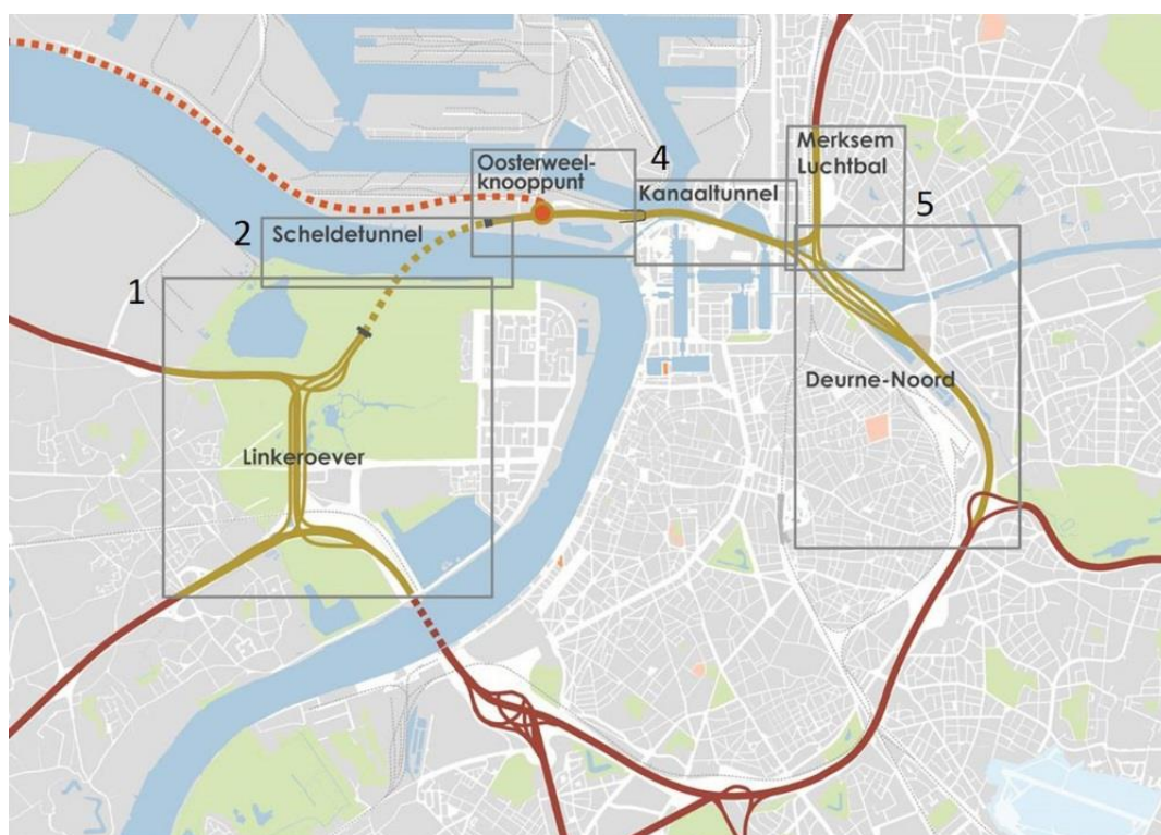
Figure 1 – Overview of the Oosterweel-connection project in which the submerged tunnel under the Scheldt, named the Scheldt Tunnel (2), is one of the five parts (RoTS).
