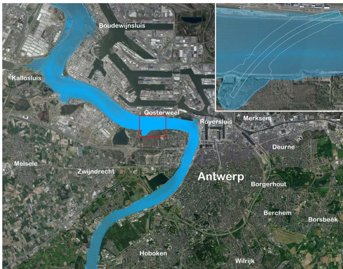
Figure 25 – Model domain of the SETMO model within the NEVLA3D model domain of the Lower Sea Scheldt; there is a close up of the model domain at the trench
