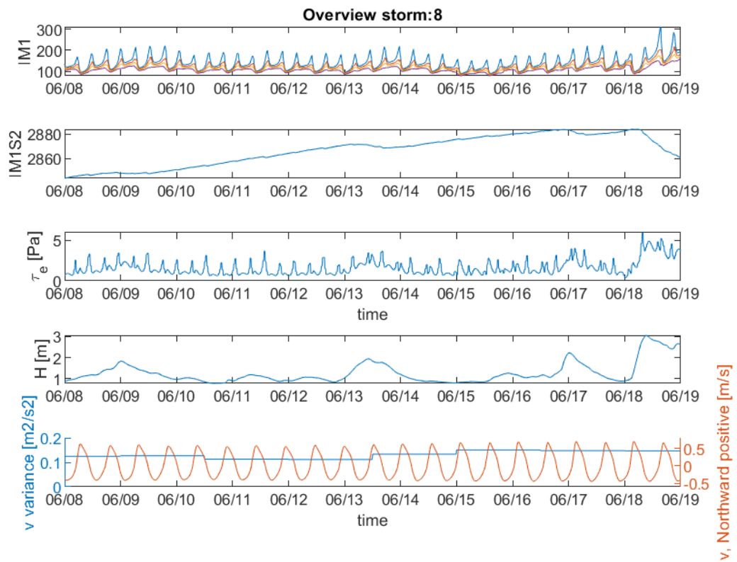
Figure 96: Storm overview from the North Sea model. These time series have a week added to either side, so are 2 weeks longer than the field data storms. From top to bottom: suspended sediment concentration, concentration in the 0.3 m thick buffer layer, shear stress, median wave height, near bed velocity and velocity variance
