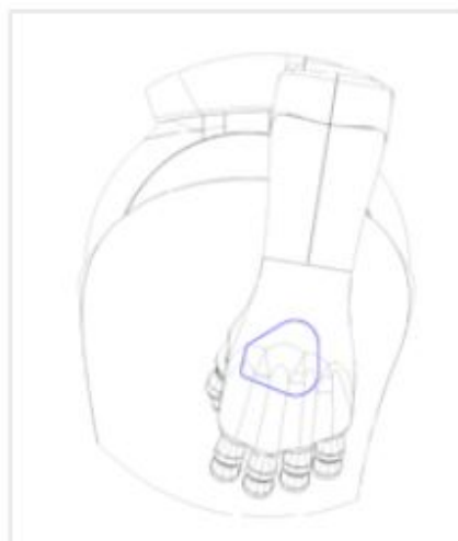
Figure C.7: Picture of the hand tactile sensors of Pepper.
