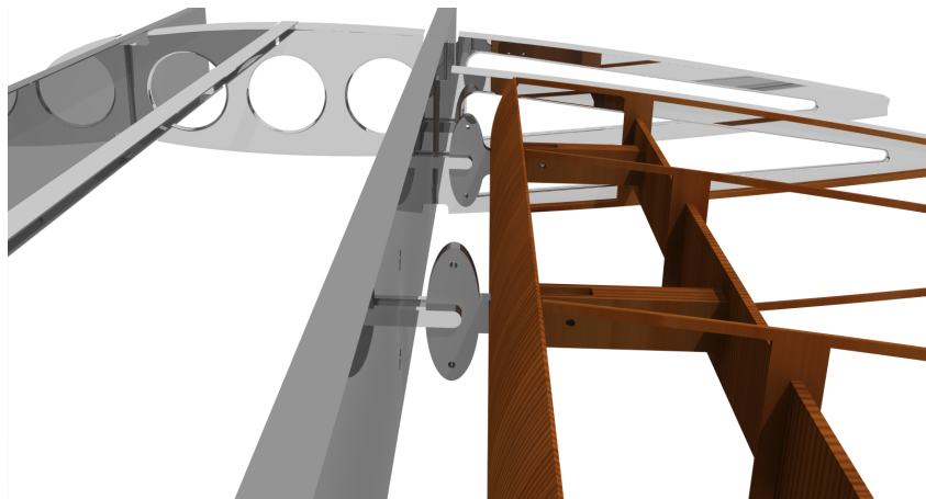
Figure 7.15: The link between the aileron control surface and the aileron hinge
