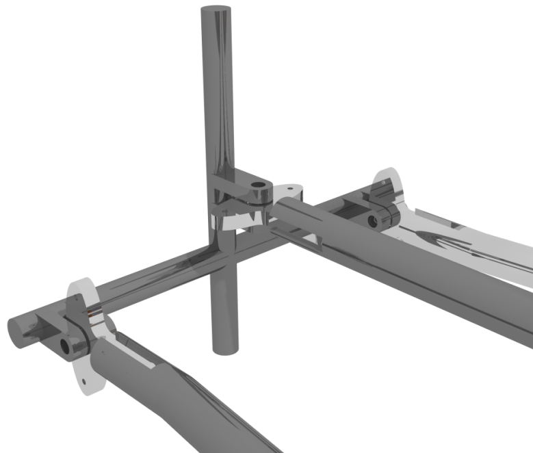
Figure 7.16: The link between the elevator and rudder control surface and their hinges
