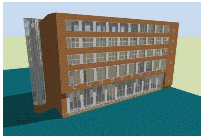
Figure 4. Model of Tower C at TU Delft developed using DesignBuilder and simulated in EnergyPlus.
