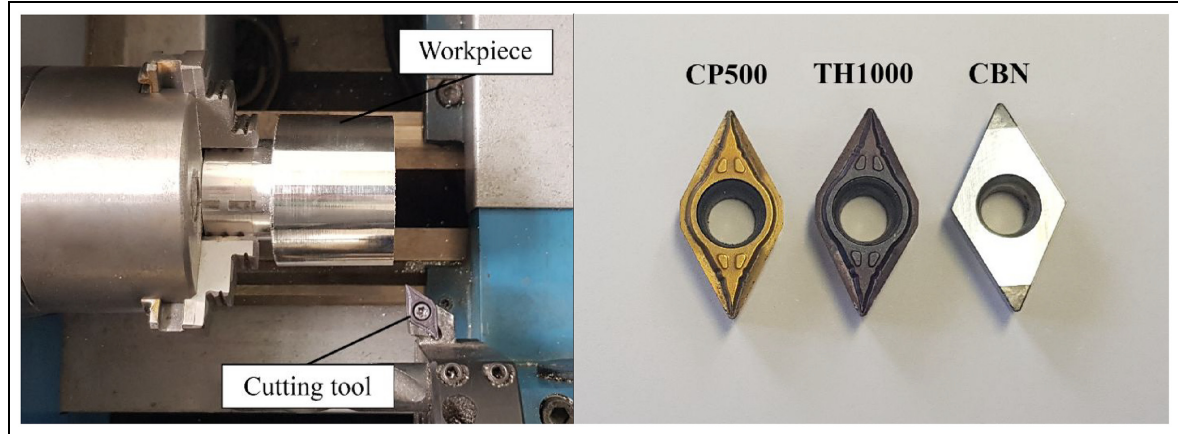
Figure 1. Machining set-up when cutting of Mg-based composites.
