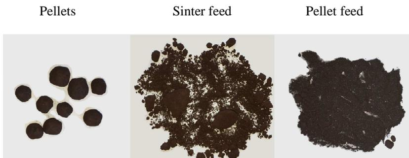
**Figure 2-1. Iron ore products with different particles sizes**
