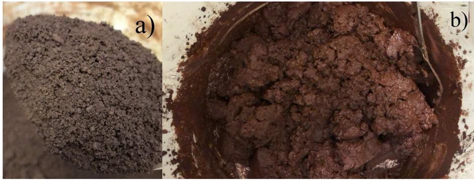
Figure 3-13. Forming large agglomerates after adding 4% extra moisture content; a)  $MC_{as,rec}$ , b)  $MC_{as,rec}+4\%$
