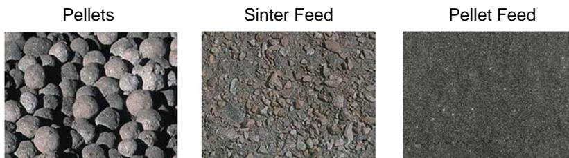
**Figure 1-6. Various size range in iron ore products; pellets, sinter feed and pellet feed [21]**
