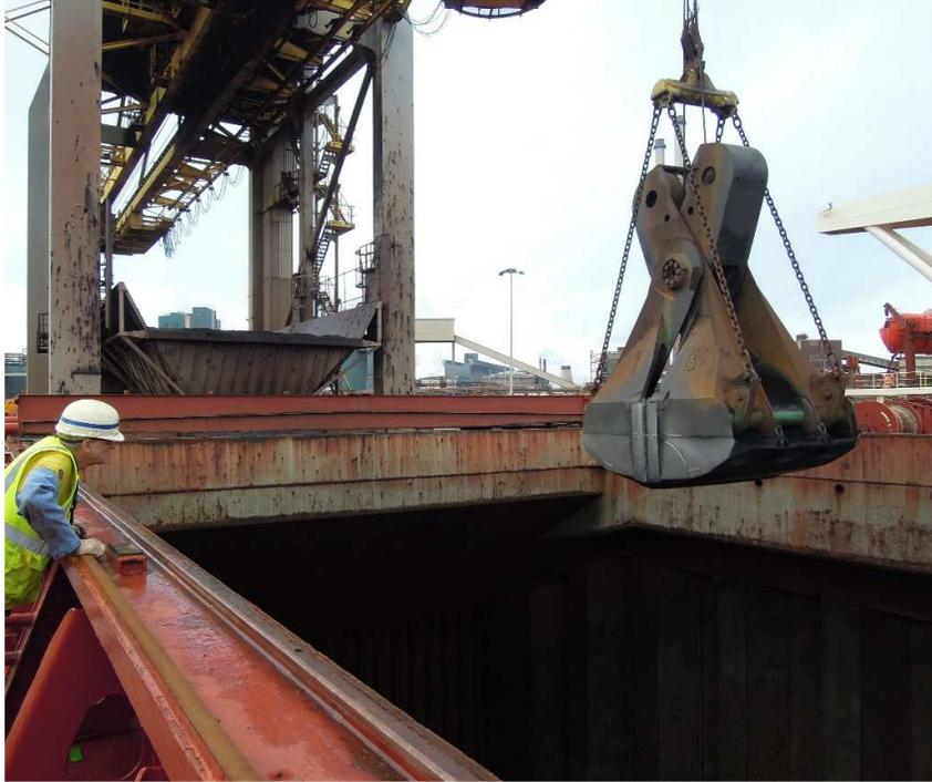
**Figure 1-1. Unloading bulk carriers at destination using grabs**
