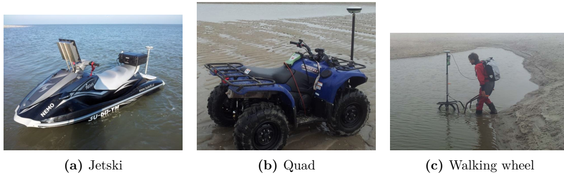
Figure C-2: Survey equipment, images: Shore Monitoring and Research (De Zeeuw, 2011–2016)
