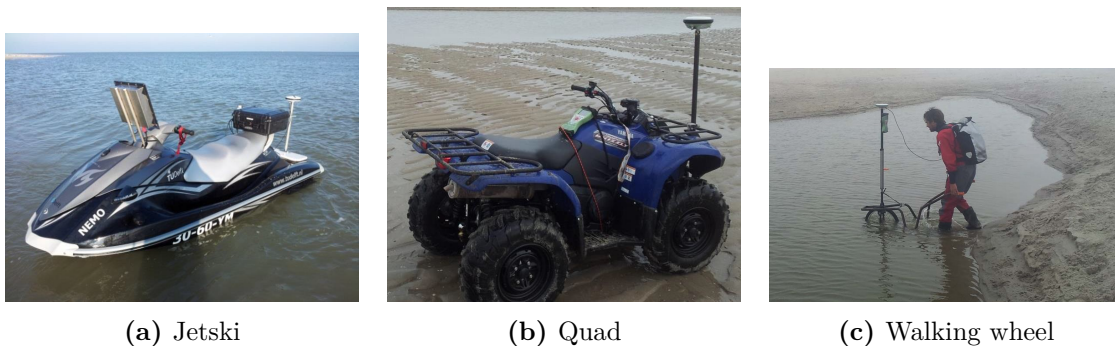
Figure 2-4: Survey equipment, images: Shore Monitoring and Research (De Zeeuw, 2011–2016)
