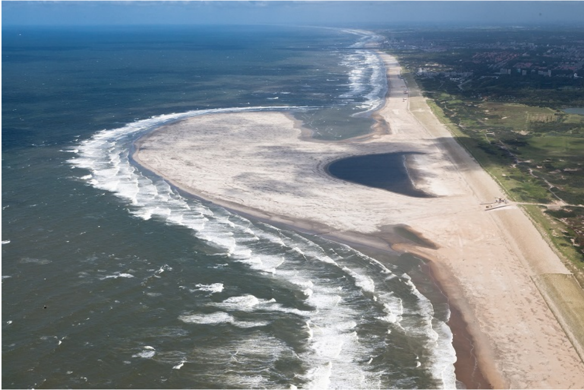
Figure 1-4: Aerial photograph of the Sand Engine peninsula just after construction in August 2011, looking to the North (Rijkswaterstaat et al., 2011).
