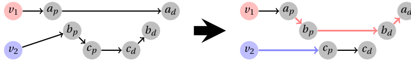
Figure 4.4: Relocate Request b is relocated to vehicle v_1 . b_p is the pickup of request b and b_d the delivery location
