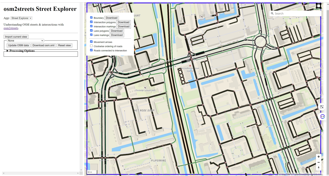
Figure 2: Screenshot of ”osm2street”, output the road polygons for a chosen region.
