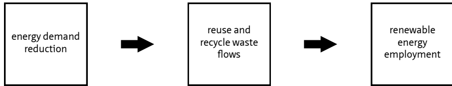
FIGURE 3.7 The new stepped approach to sustainable energy design. Adapted from Van den Dobbelaer (2008).
