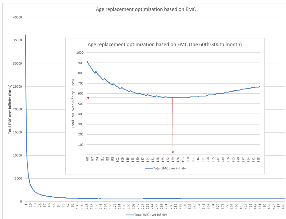
Figure 35 Output of age replacement optimization (reference case: 12-month grinding interval)
