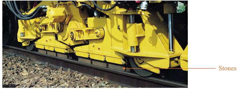
Figure 17 Grinding machine GWM 250 (Esveld, 2001, p. 352; PlasserAmerican, 2018)
