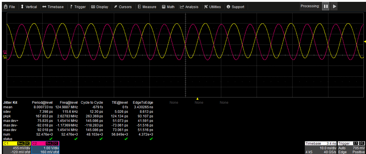
Figure D.9: A screenshot from the Teledyne LeCroy Oscilloscope of type waveMaster 813Zi-B. The transmission delay is measured on line 4. The direction: the master is measured at its oscillator, and the slave is measured at its via on the single-ended line. The bandwidth was limited to 200 MHz on both input channels. The transmission delay is expressed by the variable EdgeToEdge
