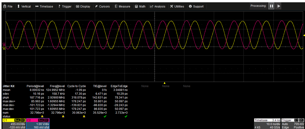
Figure D.2: A screenshot from the Teledyne LeCroy Oscilloscope of type waveMaster 813Zi-B. The transmission delay is measured on line 2. The direction: the slave is measured at its oscillator, and the master is measured at its via on the single-ended line. The bandwidth was limited to 200 MHz on both input channels. The transmission delay is expressed by the variable EdgeToEdge
