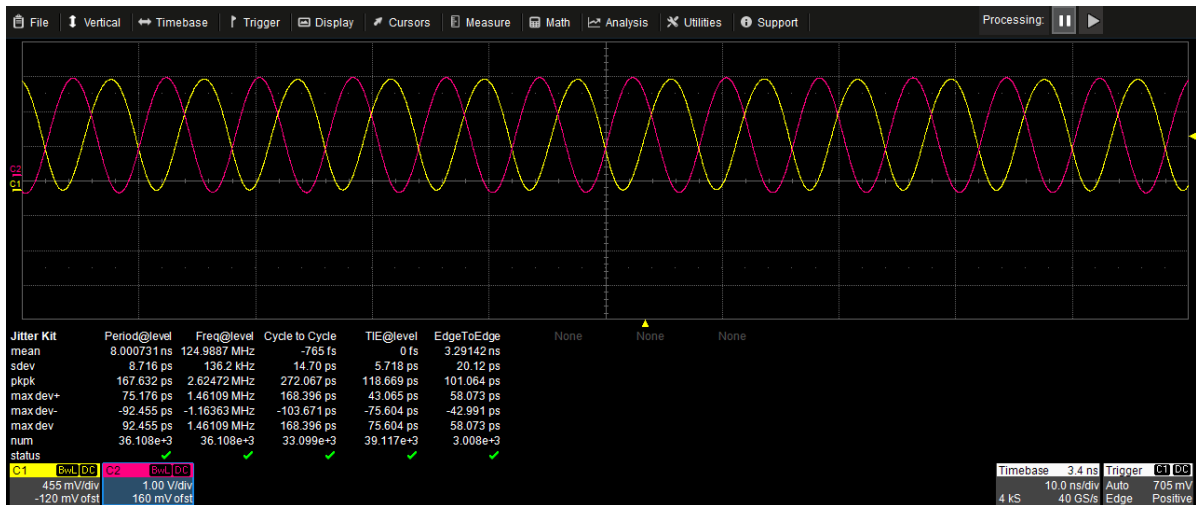
Figure D.3: A screenshot from the Teledyne LeCroy Oscilloscope of type waveMaster 813Zi-B. The transmission delay is measured on line 3. The direction: the slave is measured at its oscillator, and the master is measured at its via on the single-ended line. The bandwidth was limited to 200 MHz on both input channels. The transmission delay is expressed by the variable EdgeToEdge
