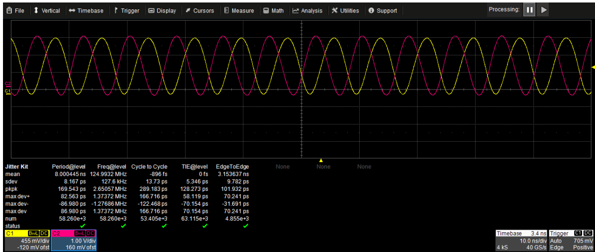
Figure D.7: A screenshot from the Teledyne LeCroy Oscilloscope of type waveMaster 813Zi-B. The transmission delay is measured on line 2. The direction: the master is measured at its oscillator, and the slave is measured at its via on the single-ended line. The bandwidth was limited to 200 MHz on both input channels. The transmission delay is expressed by the variable EdgeToEdge
