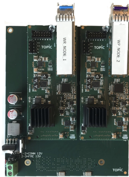
Figure 3.1: Carrier board with two Topic Artix-7 boards attached. Both boards are denoted as WR_NODE_1 and WR_NODE_2 respectively. Logically, a carrier board for an 18-port White Rabbit switch will contain 18 slots and 18 attached boards.
