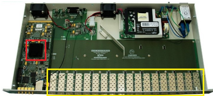
Figure 1.3: Implementation of the open-source switch from Seven Solutions. Accentuated in red, one can find the Virtex-6 FPGA. The yellow markings denote the 18 SFP-modules for the 18-port configuration of the switch [7].
