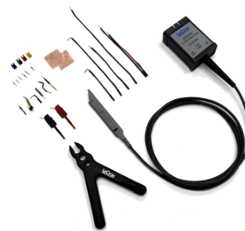
Figure 4.4: Stock image of the Teledyne LeCroy Active Probe of type ZS2500. It has a limited bandwidth of 2.5 GHz, an 8V range and an ideal input impedance of 1 M\Omega , which decreases over frequency.
