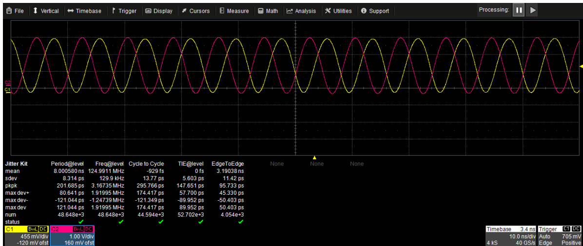
Figure D.1: A screenshot from the Teledyne LeCroy Oscilloscope of type waveMaster 813Zi-B. The transmission delay is measured on line 1. The direction: the slave is measured at its oscillator, and the master is measured at its via on the single-ended line. The bandwidth was limited to 200 MHz on both input channels. The transmission delay is expressed by the variable EdgeToEdge
