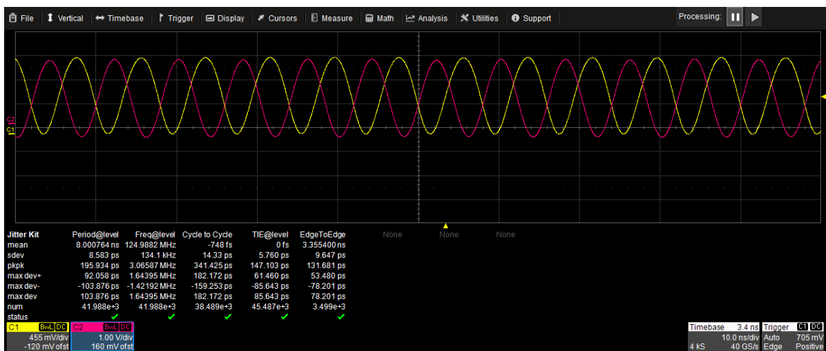
Figure D.4: A screenshot from the Teledyne LeCroy Oscilloscope of type waveMaster 813Zi-B. The transmission delay is measured on line 4. The direction: the slave is measured at its oscillator, and the master is measured at its via on the single-ended line. The bandwidth was limited to 200 MHz on both input channels. The transmission delay is expressed by the variable EdgeToEdge
