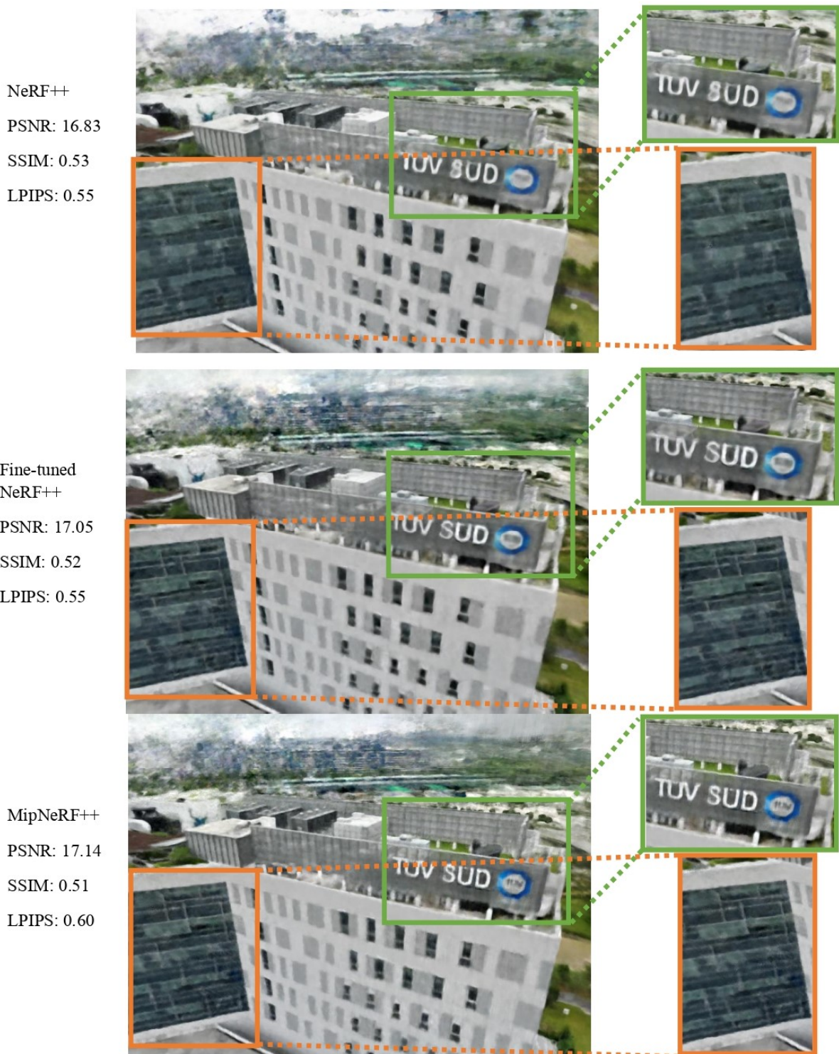
Figure 5.5: Comparison of rendering from the same view with using NeRF++, fine-tuned NeRF++ and mip-NeRF++ respectively. Fine-tuned NeRF++ and replacing NeRF with mip-NeRF can improve the ability to represent details.
