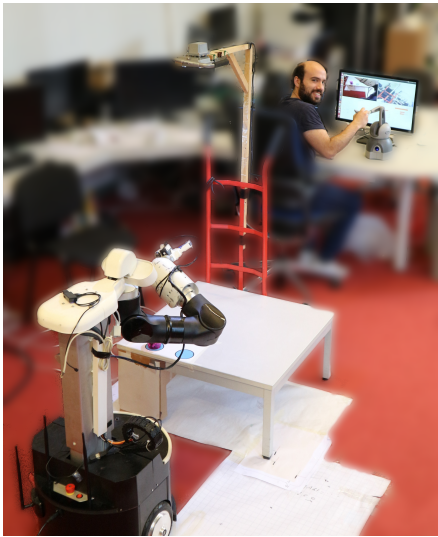
Fig. 6: Experiment setup with the operator holding the master device, Marco in front of the table with the cup and the markers and the table placed on the template. (Irrelevant background blurred.)
