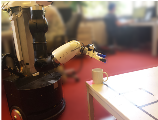
Figure 29: Base pose selected with the IHCM that resulted in a task that was not executable with telemanipulation. Irrelevant background blurred.
