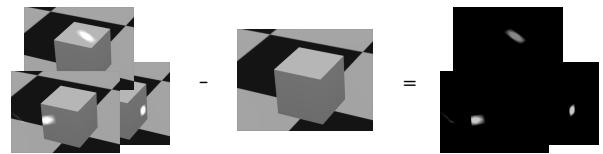
Fig. 6. The calibration step for 3 of the projector's pixels. For every pixel in the projector, a picture is taken. The picture where all projector pixels are off is subtracted from these pictures. The results are stored in the calibration matrix.
