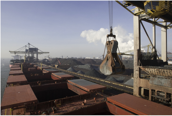
Fig. 1. Unloading a vessel with a grab at TATA Steel, IJmuiden. Courtesy of Nemag B.V.
