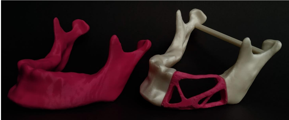
Figure 37: Additively manufactured models of the healthy intact mandible (left) and the mandible with 25% volume defect with the topology optimized implant (right).
