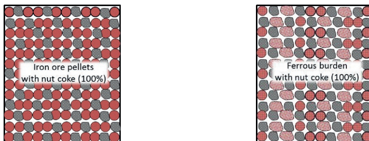
(a). Iron ore pellet mixed with 100 % nut coke (b). Ferrous burden of pellet and sinter mixed with 100 % nut coke
