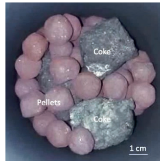
Fig. 8.4 Photograph of the sample bed from the crucible top, before experiment (pellets 10-13 mm and coke 20-25 mm).
