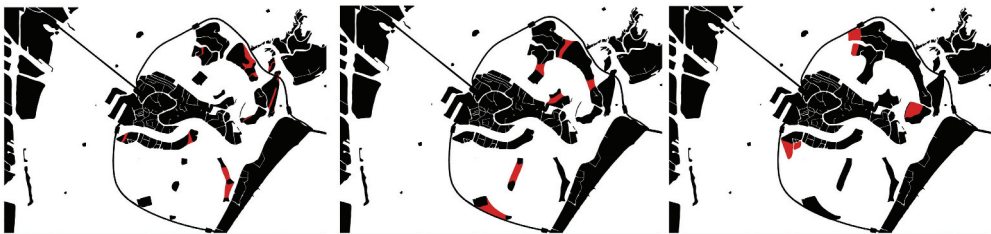
Figure 6. The symbiotic system design proposal. General plan of the dam-ring and development of the new islands (in red) through time (Buis et al. 2021).
