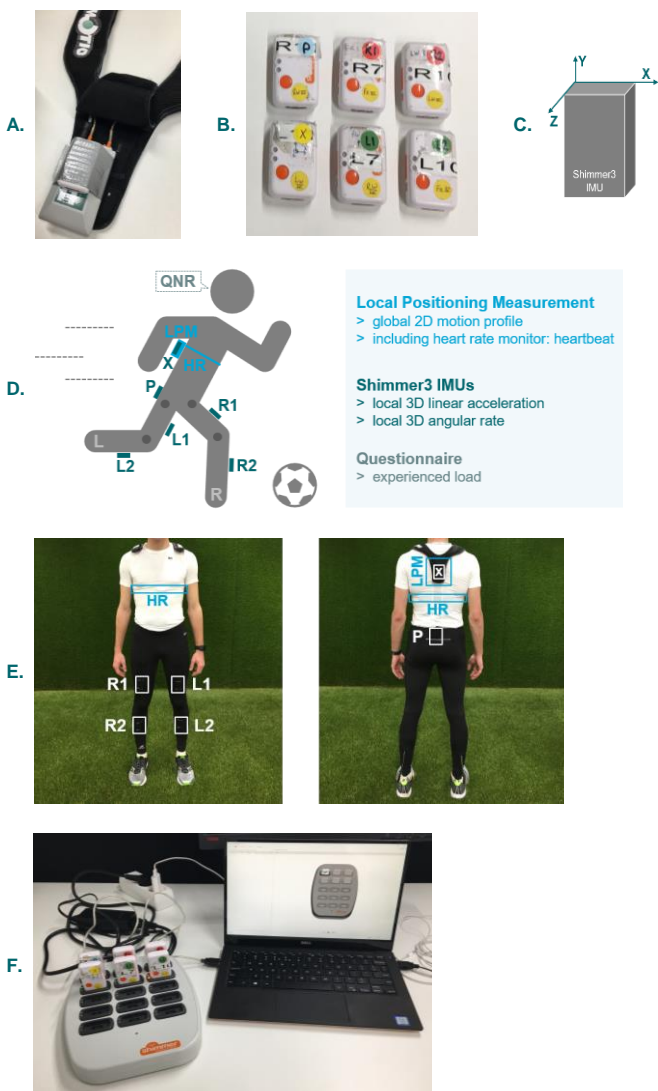
Figure 2.1 – A: LPM sensor including a reference IMU; B: All Shimmer3 IMUs; C: Internal coordinate system of Shimmer3 IMUs; D-E: Schematic representation and a picture of a participant with all measurement methods, respectively; F: Preparation and configuration of the IMUs.
