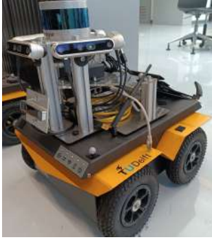
Figure 22: The LiDAR and front-facing camera of the Jackal robot are used in lab experiment
