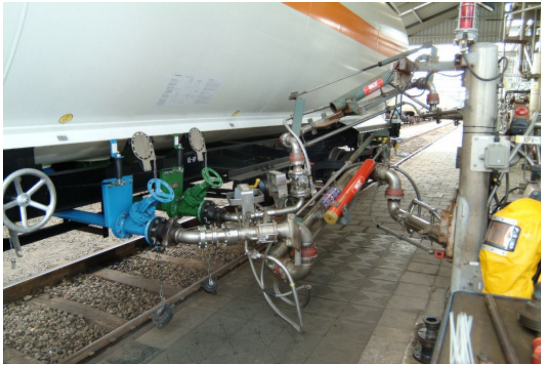
(a) An example of a loading and unloading arm for ammonia with a train [35]
