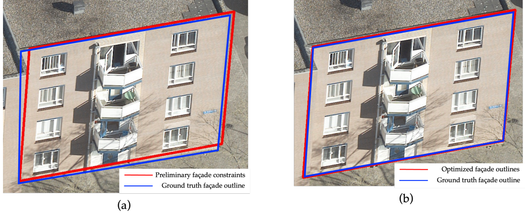
Figure 4.6: Comparison of initial projection result and optimization result
