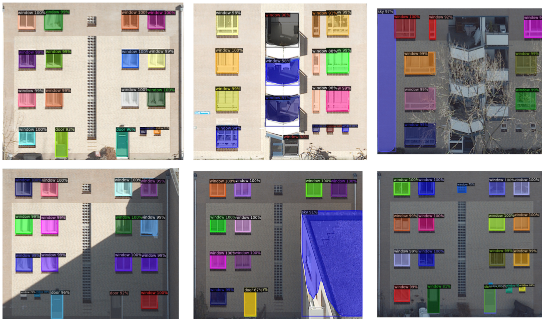
Figure 6.5: Successful openings detection result using Mask R-CNN
