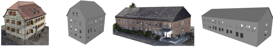
Figure 3.6: LOD3 model reconstruction (Figure from [Huang et al. [2020]])
