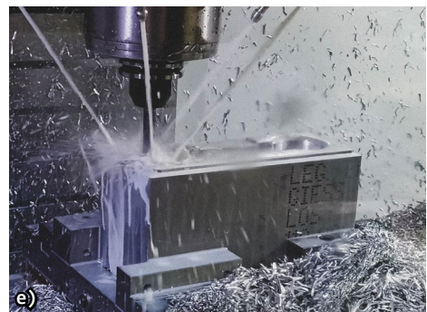
Figure 58.- Delft Engine manufacturing shoots. a) Experiencing for the first time the motion of the full armature assembly; b) CNC milled components; c) Moritz tapping holes; d) Delft Engine concept design; e) CNC milling of the motor mount components using the Dream Hall's facilities
