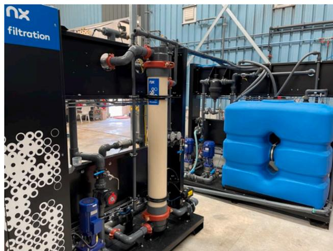
Fig. 1. Dnf 40 membrane module (nx filtration bv, Enschede, NL).
