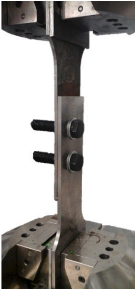
Fig. 5. Fatigue test on single shear bolted connection.
