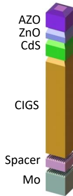
Figure 3.4: Modified model with the synthetic dielectric spacer layer. Thicknesses of different layers (in nm) from top to bottom are as follows: 250, 60, 70, 1600, d and 320. The thickness d of the spacer layer was varied between 20 nm and 170 nm.
