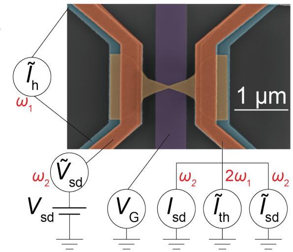
ately after the junction formation, the system is cooled down to T=2 K for stability and sharp Fermi-Dirac distributions for the thermoelectric study.
