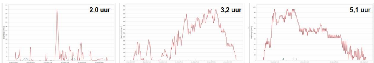
Figure 16 Graphs depicting progression of total delays of trains with various processing times (2;3.2;5.1 hrs resp.).
