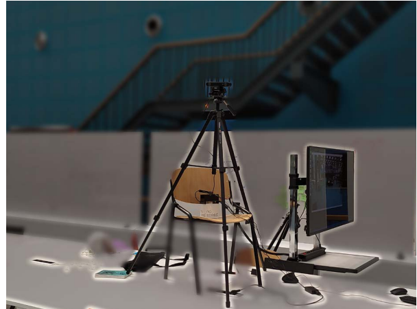
Figure 24: Setup used to perform feasibility study of the Zed 2 camera
