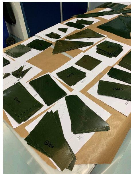
(b) Some of the patches and sub-patches of the blended laminate after cutting.
