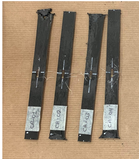
Figure 8.1: The 0° compressive specimens after testing.
