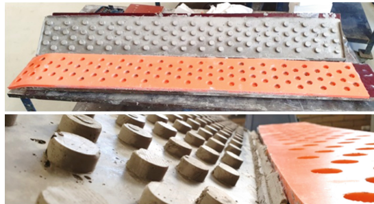
Fig. 2. Shearkeys in profiled SHCC laminates.
