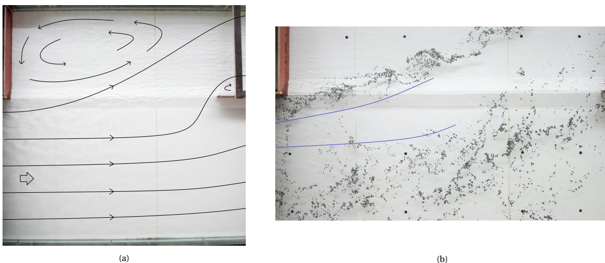
Figure 4.1: Top views of the flume: (a) top view of the flume with hand-drawn flow lines and (b) top view of the flume during PIV measurements with floating particles in the experiment A2 with discharge Q = 35 \text{ m}^3/\text{s} and downstream weir heights: h_s = 60 \text{ mm} in the sheltered channel and h_s = 80 \text{ mm} in the main channel. The blue curves indicate the area where the flow diverges in the upper layer.
