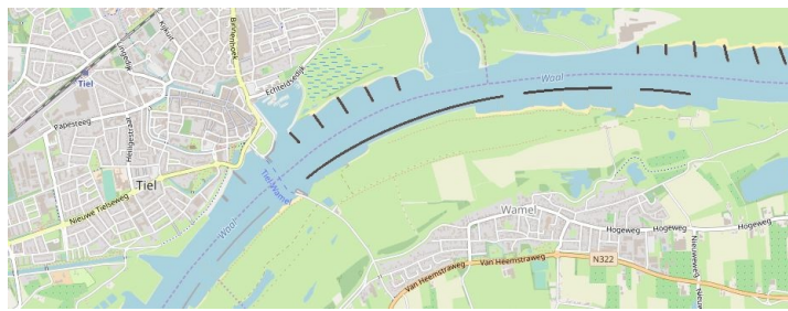
(a) Map with the longitudinal training walls in the river Waal near Wamel [EduGIS]
