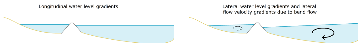
Figure 2.4: Sketch of the channels with different longitudinal water level gradients in the channels (left) and different lateral water level gradients in the channels and lateral velocity differences due to helical flow in river bends (right) based on Van Linge [2017]
