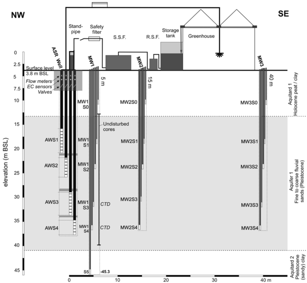
Figure 3-2: Set-up of the ASR field trial. MW = monitoring well, CTD = electric conductivity, temperature, and pressure datalogger, R.S.F. = rapid sand filtration, S.S.F. = slow sand filtration.
