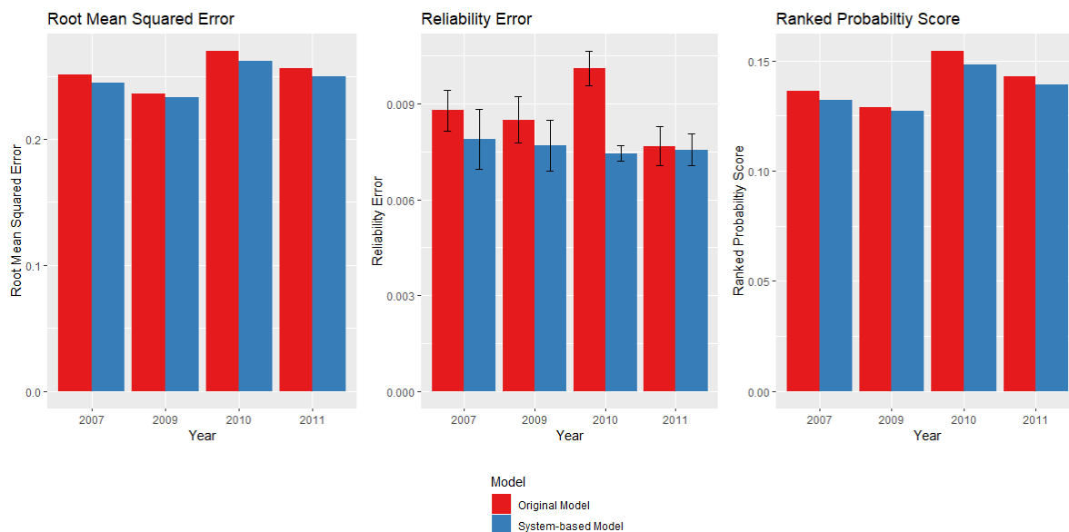
Figure 3.22: RMSE, Reliability and RPS error metrics. The output-based original model in red is compared against the proposed system-based model in blue.
