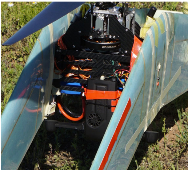
FIGURE 35 The S.L.A.M.dunk vision system was mounted on the DelftaCopter looking away from the main rotor. In hovering flight, this means the camera has a perfect view of the ground, and in forward flight the camera looks backwards. Thanks to the wide field of view fish-eye lenses, the camera can nevertheless still look vertically down during forward flight
