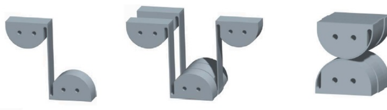
Figure 4.3: Three phases in the manufacturing of the CORE hinge, with the rightmost depicting the final product [5]
