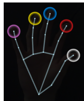
Fig. 2. Visualization of the player's hand, as captured in PIZZICATO: each finger has its own color, used by a node to indicate which finger it should be pinched with.
