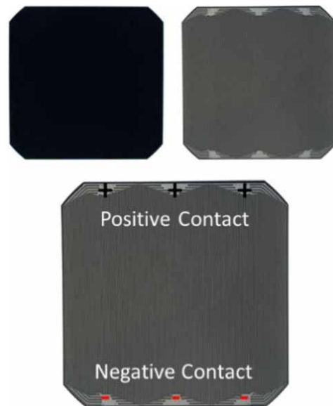
FIG. 5.3 Front and rear representation of an Interdigitated back-contact cell
