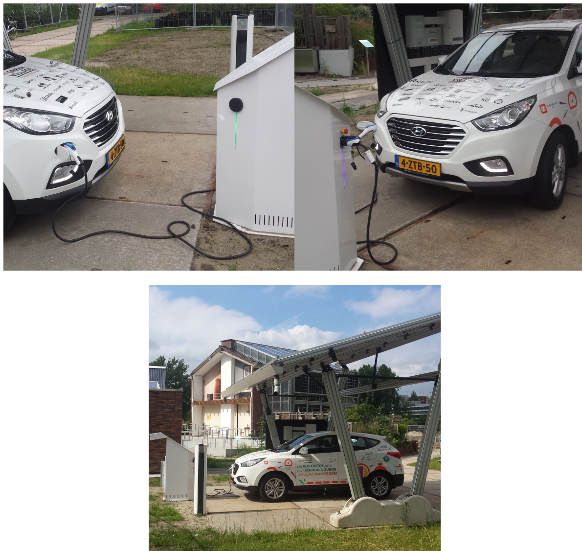
Figure 1.6: Hyundai ix35 Fuel Cell Electric Vehicle operating in V2G mode in a actual V2G set-up at the TU Delft Green Village site
