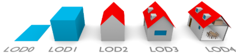
Figure 1.2.: The five Level of details of the OGC CityGML 2.0 ( taken from Biljecki (2017))
