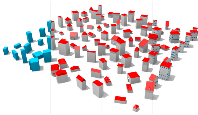
Figure 2.6.: Composite rendering of a dataset in four LODs (1.2, 2.2, 2.3, and 3.3)(taken from Biljecki (2017))
