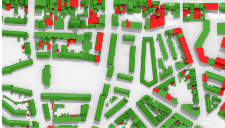
Figure 2.18.: Orientation of roof surfaces, where green is correct, red is wrong (taken from Biljecki et al. (2016a) )
