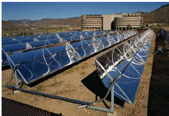
Figure 4-19 : Concentrating solar collector (Tyagi et al., 2012)
