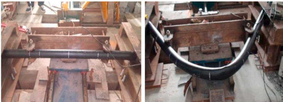
Fig. 12. MFSP specimen before and after bending.
