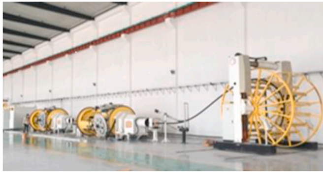
Fig. 1. Pipe coiled in the reel drum.
