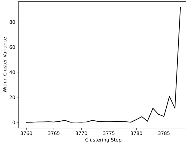
Figure 4: Zoomed in elbow plot for the difference in the within-variance of the clusters after each clustering step using an agglomerative hierarchical clustering algorithm applying the ward distance metrics(weighting = 30)
