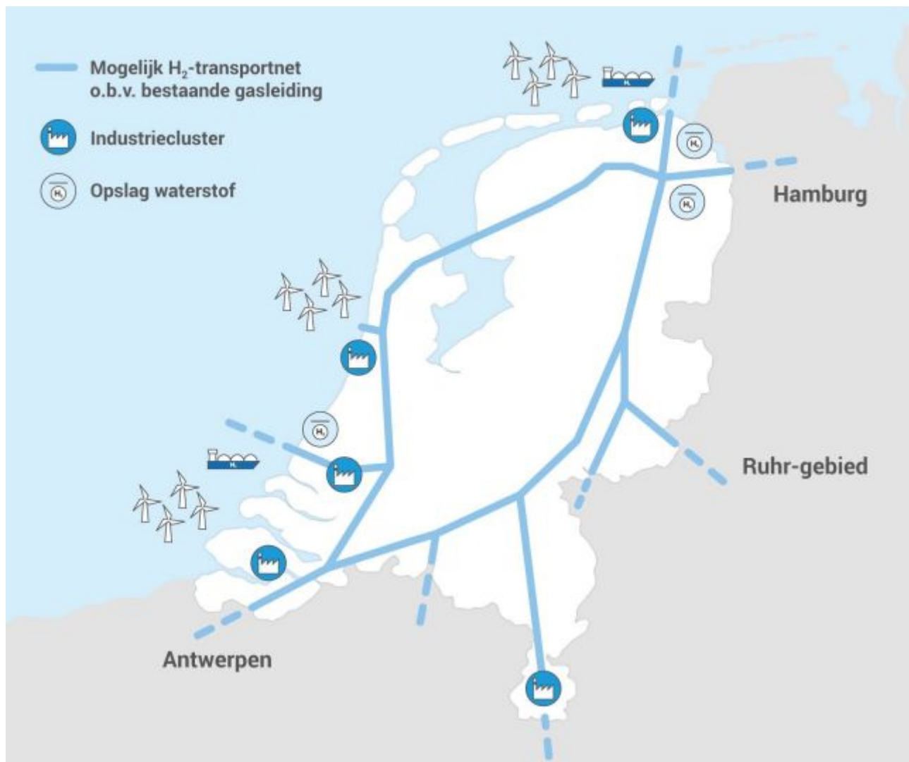
Figure 30: Schematic depiction of Dutch HyWay 27 project for hydrogen interconnection based on existing natural gas pipelines (Gasunie, 2020)
