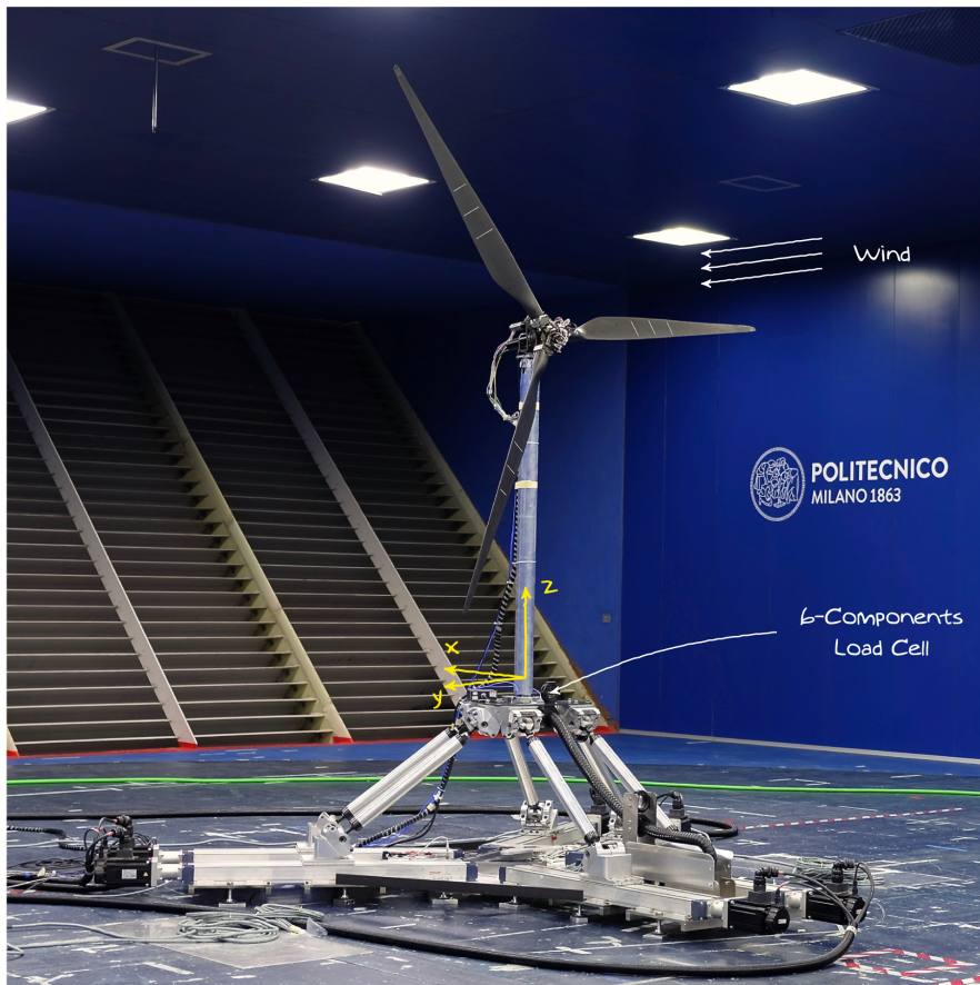
Figure 2.2: Set up of a scaled wind turbine with 6DOF 'HexaFloat' robot for HIL testing in the wind tunnel at Politecnico di Milano [69]
